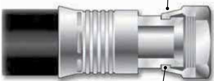
Swivel joint sensitive to over-torquing
